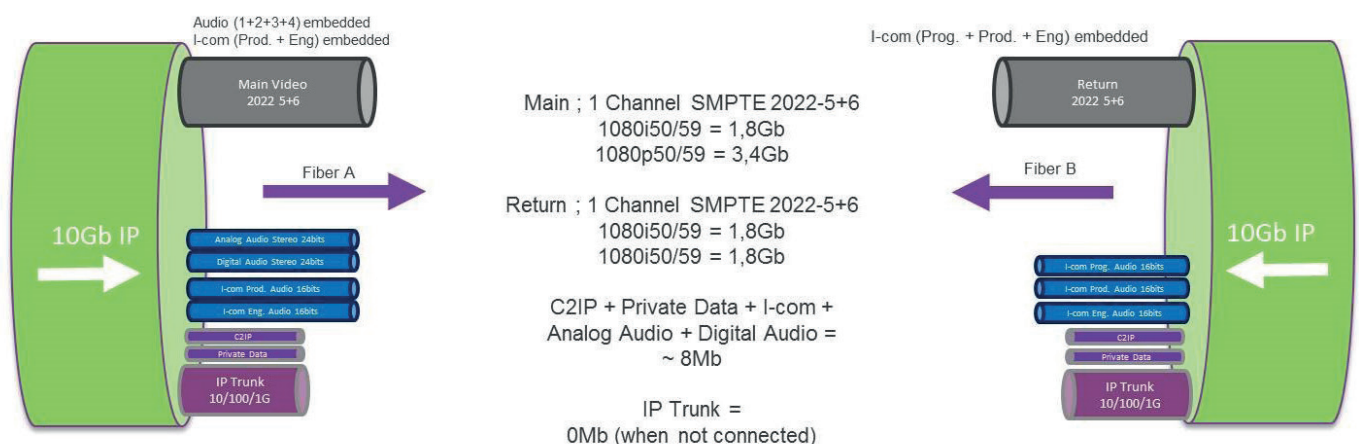
FIGURE 3: XF TRANSMISSION PROTOCOL
