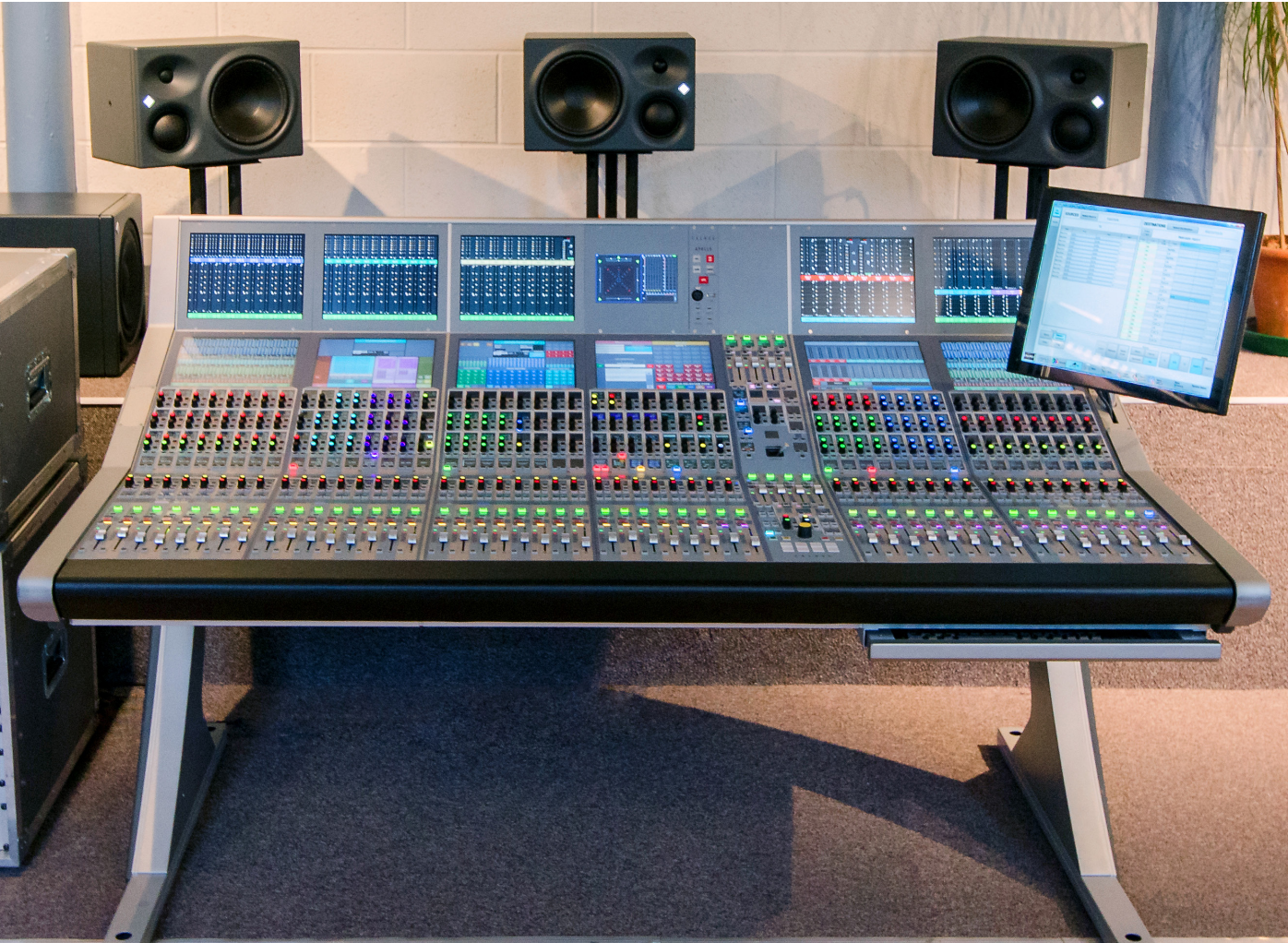
48 Fader Calrec Apollo Console with 5.1 monitoring system at Hebden Bridge
